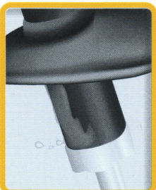
Fluid leaks from shock or strut body
